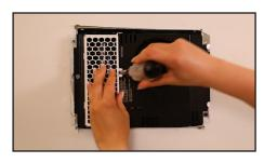
9. Install the front grill using the screw.
