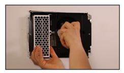
4. Remove the grill that is secured with a screw.
